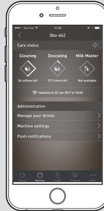
As soon as the Wi-Fi has been successfully set up, the machine's Wi-Fi indicator light will light up permanently. The App will direct you to the details page for your Qbo machine. Here you will see the current maintenance status, and you can rename the machine or change settings.
