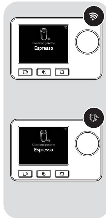
If the Wi-Fi indicator light lights up permanently, the machine is already connected to a Wi-Fi network.
