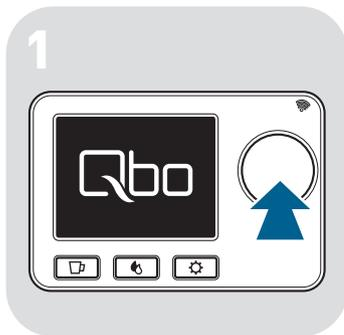
▷ Press the dial to switch on the machine.
